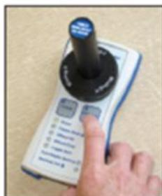
A fast optical communication interface with the Reader allows typical study samples of ~10,000 to offload in 7 seconds. The Reader also indicates if your data logger battery or memory is low.
